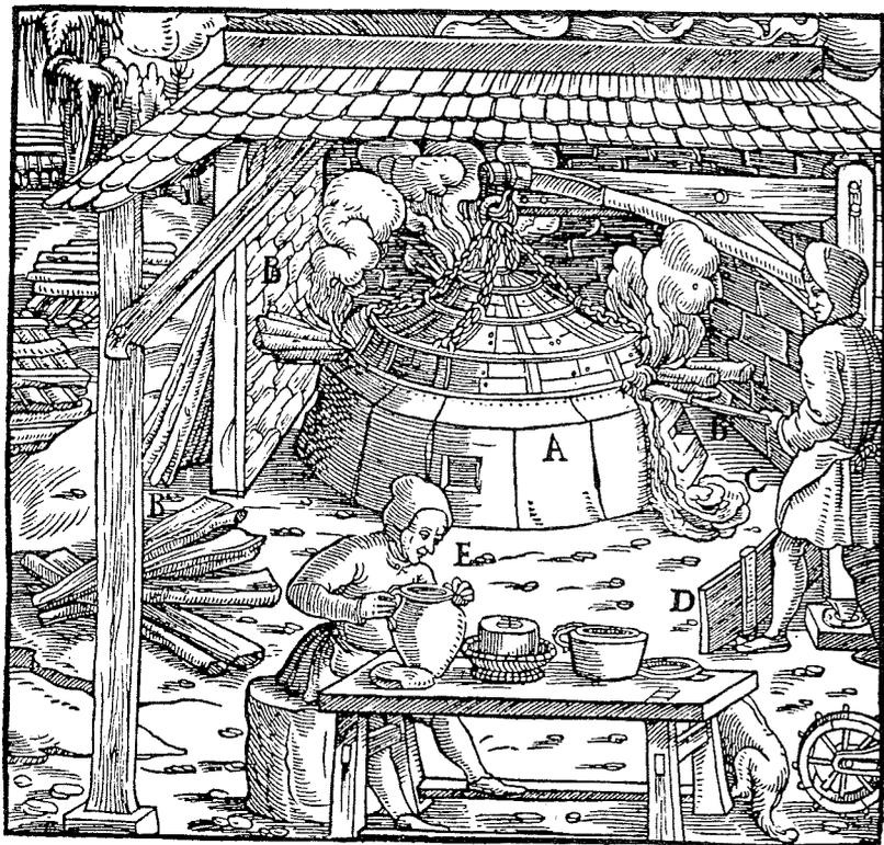
A: Fourneau B: Le bois de chauffage C: La litharge D: Planchettes
